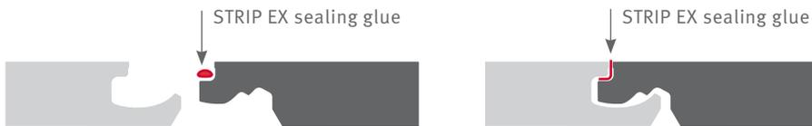
Additional exposure to moisture in commercial areas must be anticipated. Therefore it is required to use the specially designed STRIP EX sealing glue for commercial area installations. Apply the STRIP EX sealing glue to the top of the tongue on the short and long edge. The glue should ooze out along the complete long and short edge after the panels have been connected together. It is easy to remove excess sealing glue from the surface either immediately or after a short drying period.
